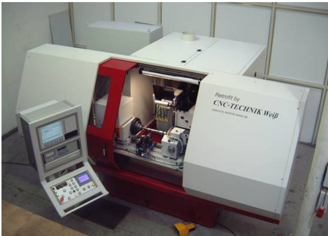
Fig 3.: A retrofit machine of CNC-Technik Weiß cannot be distinguished from a new circular grinding machine
