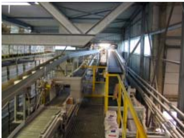
Fig 2.: The conveyor lines for full pallet transport
