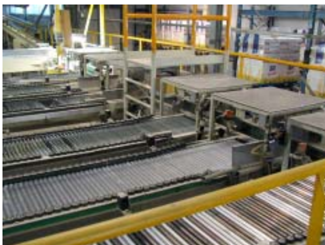
Fig. 3: Accumulating roller conveyors of the multi-palletiser
