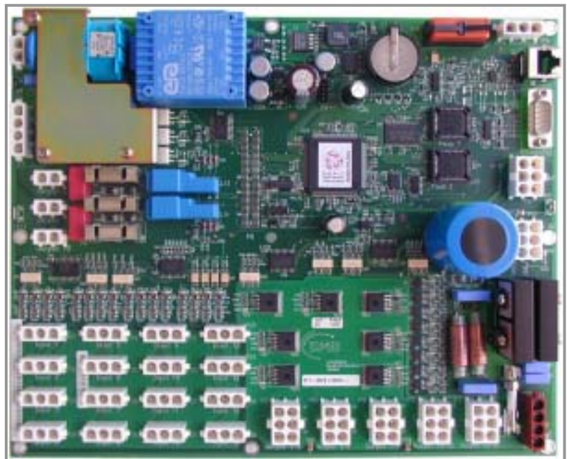
Fig.: The pc board of the SMB ST1 control system
